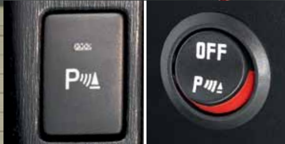
Cancellation switches You can switch off the parking aid sensor alarms when not required.
