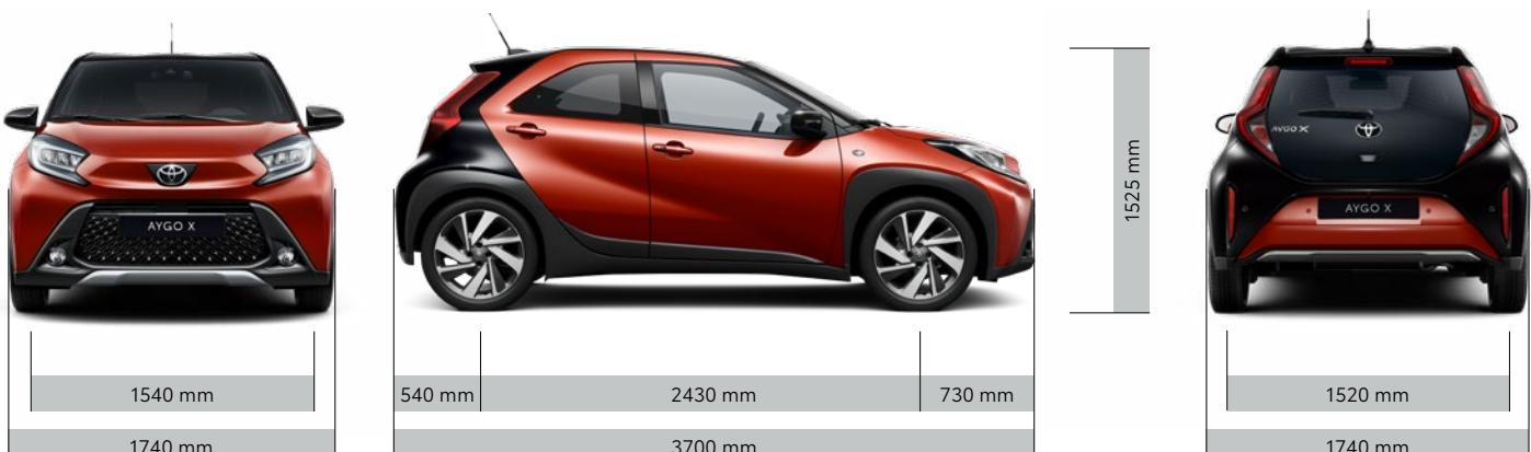
The technical drawings illustrate the dimensions of the Toyota Aygo X. The front view shows the overall width of 1740 mm. The side view provides a comprehensive look at the car's proportions: length 3700 mm, width 1540 mm, and height 1740 mm. The rear view highlights the height of 1525 mm and the overall width of 1740 mm.
